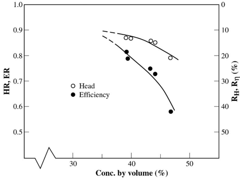
Figure 3. Reduction in head and efficiency at high solids concentrations for a sand with  $d_{50} = 0.35$  mm and an all metal pump (impeller diameter = 0.63 m). From Wilson et al.2006. The increasing power requirement corresponding to  $ER/HR <1$  in Figures 2 and 3 can be represented by a factor,  $c >1$ , in eq.3 (Sellgren et al.2002).
