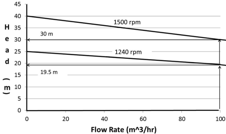
Figure A2. Pump head curves for 1240 and 1500 rpm approximated as straight lines for the considered flow rates and heads. To maintain the operating point at 19.5m for 100 m<sup>3</sup>/h the pump has to develop 1500 rpm to account for the derating effect.
