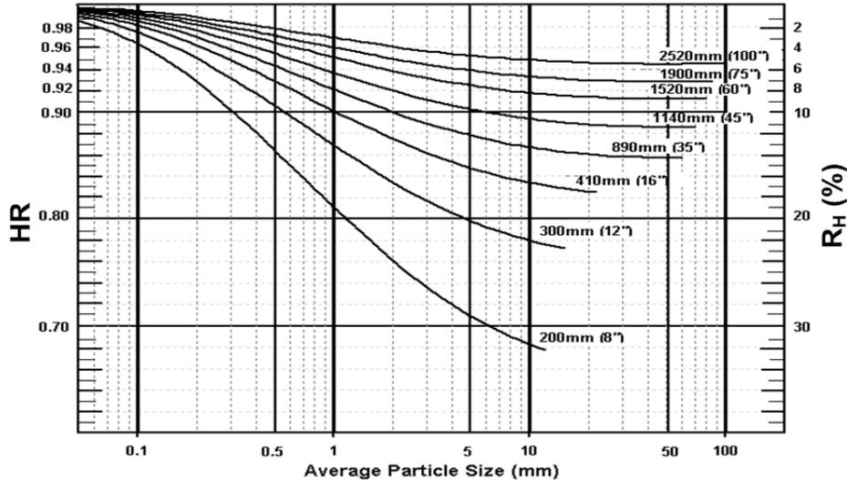
Figure A1. Generalised solids-effect diagram for pumps of various sizes (impeller diameters). For solids concentration by volume 15% with relative density of solids, 2.65, and a negligible amount of fine particles smaller than 75micron. From ANSI/HI (2011).
