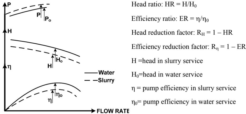
Figure 1. Sketch defining the derating in head and efficiency of a centrifugal pump transporting a settling type of slurry.  $P$  is power requirement in slurry service and  $P_0$  is power requirement in water service.
